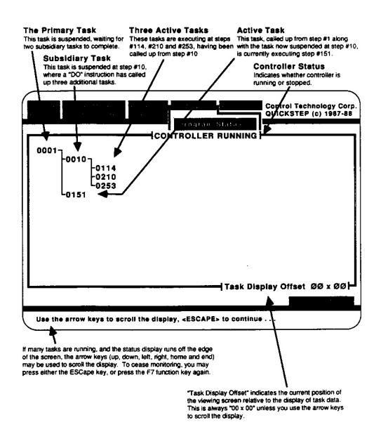
detected by the controller, resulting in a "software fault" and a subsequent automatic shutdown. In this case, Program Status monitoring will provide you with a specific error message, while highlighting the step number in which the fault was first detected.
